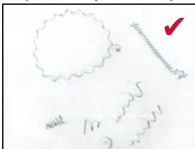
STX insert (with chipbreaker)
