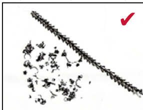
STX insert (with chipbreaker)
