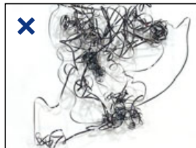
Competitor (with no chipbreaker)
