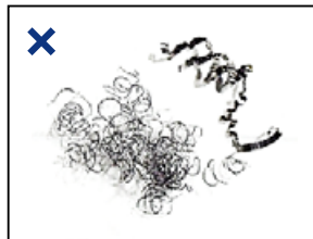
Competitor (with no chipbreaker)
