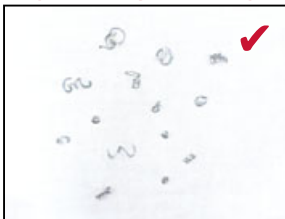
STX insert (with chipbreaker)
