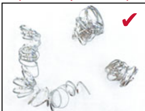
STX insert (with chipbreaker)
