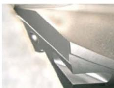
Sharp and uncoated cutting edge design prevents built-up edge and provides good chip evacuation during drilling of non-ferrous metal.
