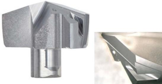
Sharp and uncoated cutting edge design prevents built-up edge and provides good chip evacuation during drilling of non-ferrous metal.
