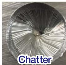
**P** Tool :  $\phi 13$  mm, L/D = 12 (No pilot hole)
