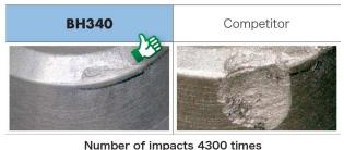
Alloy steel (HRc62)  $v_C$ =75m/min, f=0.1mm/rev,  $a_D$ =0.1mm, Heavy interrupted
