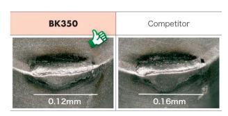
Ductile cast iron (FCD600)  $v_{C} = 300 {\rm m/min}, f = 0.1 {\rm mm/rev}, a_{D} = 0.2 {\rm mm} \quad {\rm After \ processing \ 4Km}$
