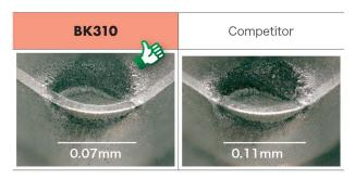
Gray cast iron (FC300)  $v_{C} = 500 {\rm m/min}, f = 0.3 {\rm mm/rev}, a_{D} = 0.3 {\rm mm}$  After processing 3 Km
