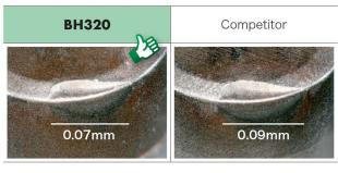
Alloy steel (HRc62)  $v_C$ =150m/min, f=0.1mm/rev,  $a_D$ =0.2mm, Continuous
