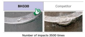
Alloy steel (HRc62)  $v_C$ =150m/min, f=0.1mm/rev,  $a_D$ =0.2mm, Heavy interrupted
